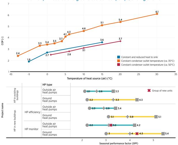
Figure 2.2 COP for heating for air source heat pumps in Switzerland and annual SPFs in Germany: Air source and ground source heat pumps, existing and new
